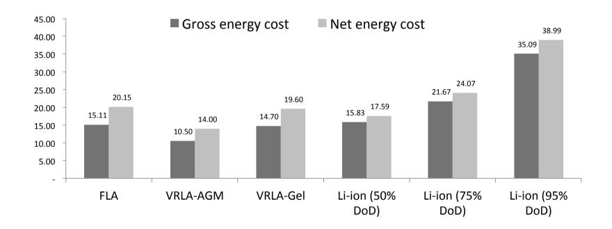
Cost per kWh delivered by the battery
